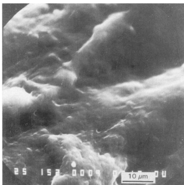
Figure 4 Scanning electron micrographs of PSS resin. Regulator concentration C = 1.05 \text{ mol/l}^{-1} .
